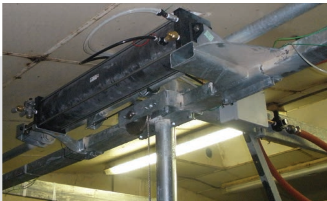
The large air cylinder on the exit gate with remote-mounted reserve air tank, provides smooth and rapid lifting of the exit gate in only four seconds - the fastest in the industry. A single cylinder can lift up to 20 stalls.
