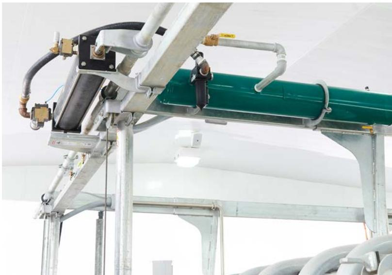
*The large air cylinder for the exit gate, with remote-mounted reserve air tank, provides smooth and rapid lifting of the exit gate in only four seconds — the fastest in the industry. A single cylinder can lift up to 20 stalls.*
