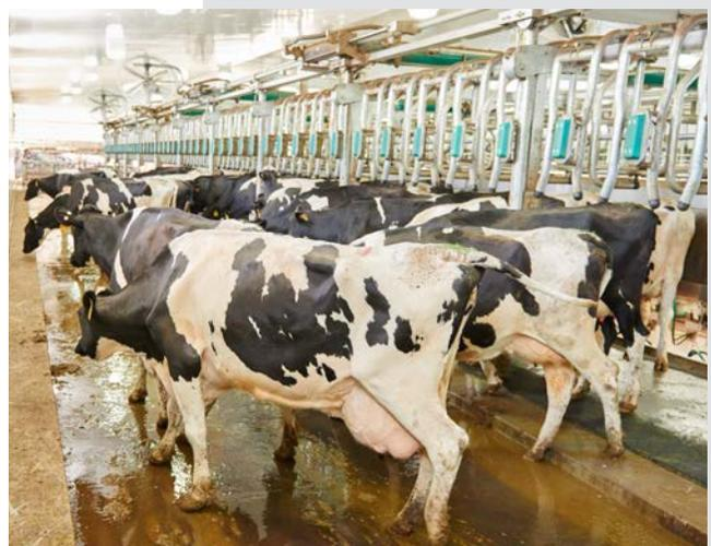
The heavy-duty construction of the Magnum 90i™ VL is designed for the demands of large, commercial dairies, milking 24 hours a day. The vertical lift exit gate allows for fast exit, increasing efficiency and turns per hour.
