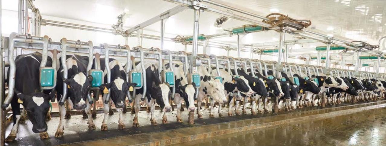
*The Magnum 90i™ VL stall automatically provides pre-indexed cow positioning. This results in proper udder presentation, and optimizes operator procedures, including unit attachment to improve throughput.*
