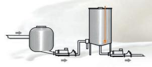
The single float 55" analogue probe can be programmed to optimize the milk/wash reservoir.
