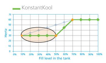
Compared to a basic switching shaft, KonstantKool keeps the pump speed low for as long as possible.
